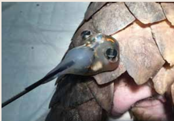
VHF tag attached on a pangolin scale for tracking via radio telemetry Photo: Paige Lee/WRS
